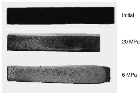
Fig. 5. Photograph of SHS samples compared with the initial compact (mixture B,  $P_{\text{comp}} = 300$  MPa).
